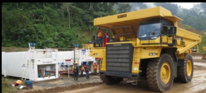
A double wall tank is exactly as the name suggests. The tank literally has two walls, welded together and if the first wall ruptured from the inside, there is a second wall that stops the entire tank from leaking into the environment.
